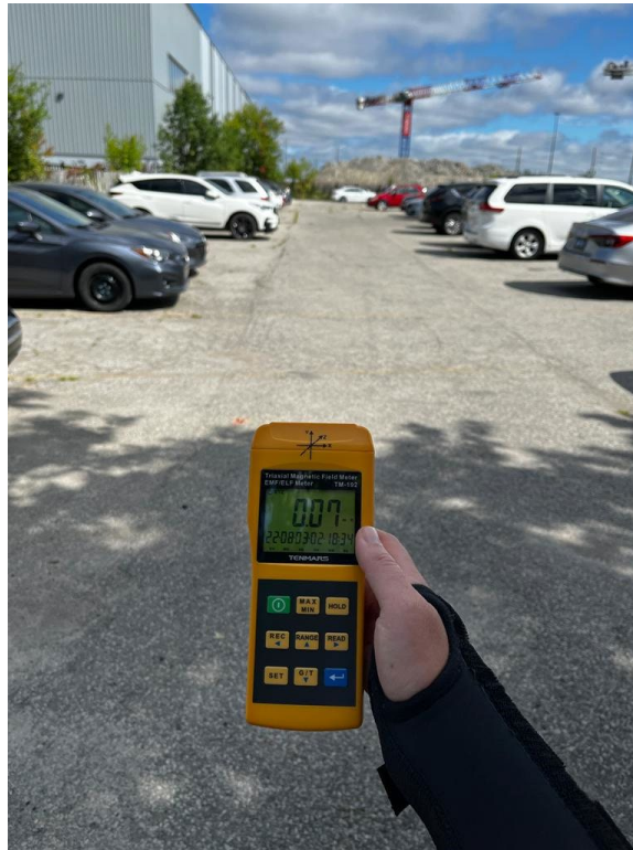
PHOTO #7: A.C. magnetic field measurements almost non-existent throughout the property.
