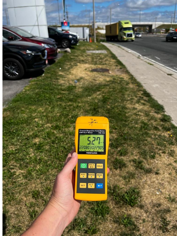
PHOTO #1: Elevated A.C. magnetic field readings recorded along Dufferin St near the North York Hydro Vault.
