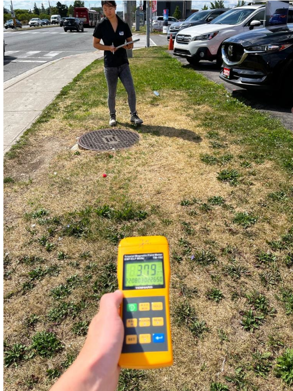
PHOTO #2: A.C. magnetic field readings depleted with distance from North York Hydro Vault.
